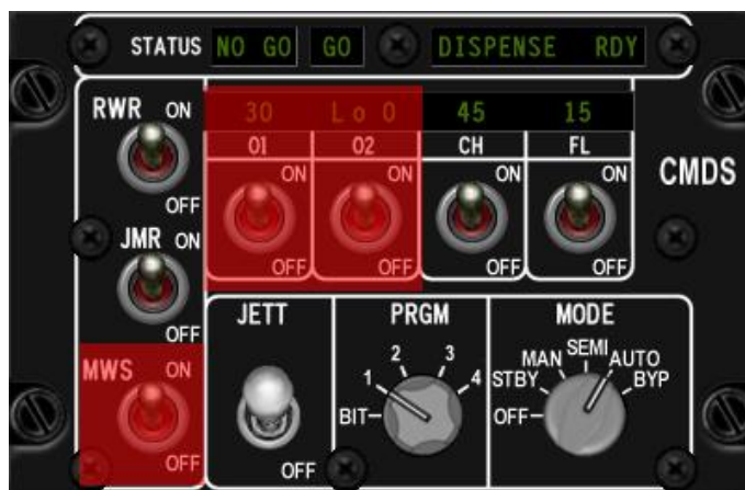
Figure 54 CMDS Cockpit Control Unit (CCU)
