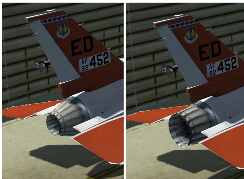
Performing the SEC check, nozzle closing & opening
